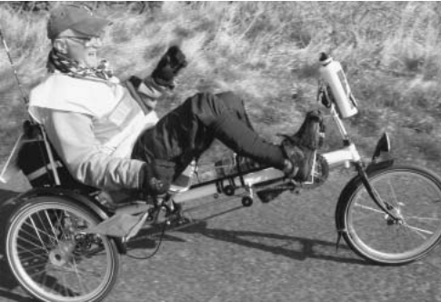
ABOVE: The Hase Kettwiesel is well-suited to special needs use, and a hand-cranked version is available along with many adaptations. Several can be linked together for ‘tandem’ use too if required.
