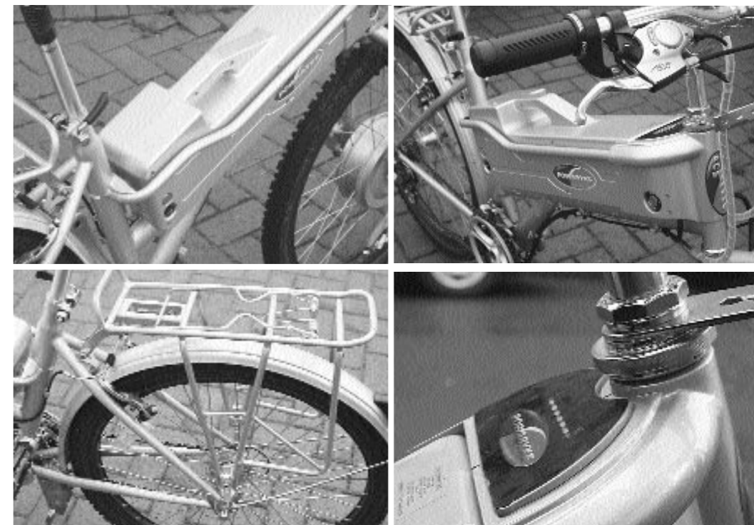
TOP LEFT: The 12kg lead-acid battery powers the bike for up to 20 miles, and can be recharged on or off the bike
