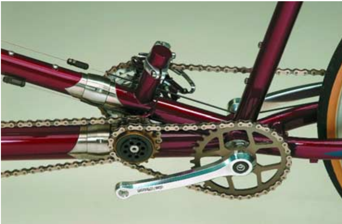
ABOVE: The unique da Vinci drivetrain: the extra shaft lets either rider freewheel at will
