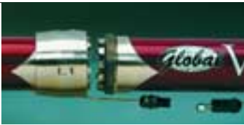
RIGHT: S&S couplings split the bike for transport, yet lock up rigid for riding
