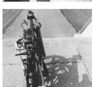
"The frame is a modified Brompton one, in steel and titanium. The main frame hinge has been done away with, which means that while the folded package isn't so compact, it's a convenient long thin shape - and the whole bike can be made lighter.
